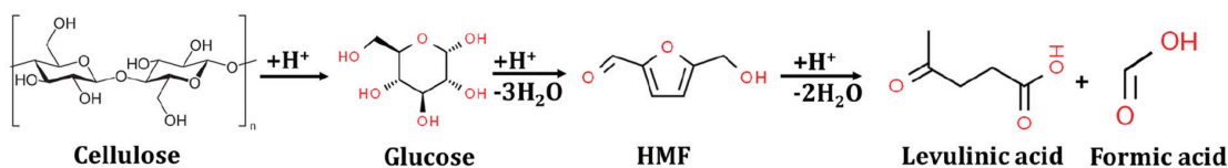
Figure 3. Products of acid hydrolysis of cellulose. HMF, hydroxyl methyl furfural.
