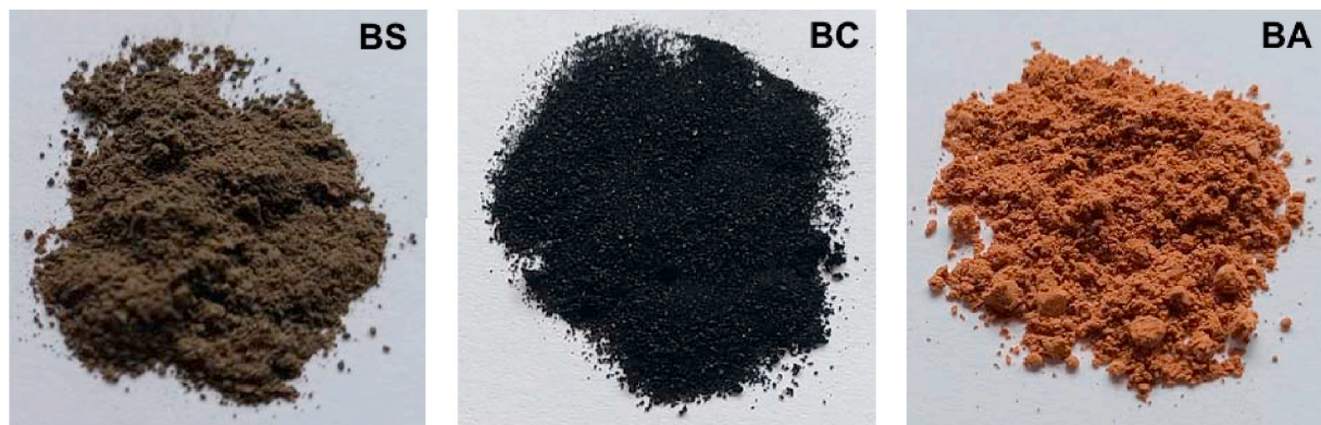
Fig. 2. Photographic images showing the physical appearance of biosolids (BS) – earthy green, biochar (BC) – black and bioash (BA) – brown. (For interpretation of the references to colour in this figure legend, the reader is referred to the Web version of this article.)
